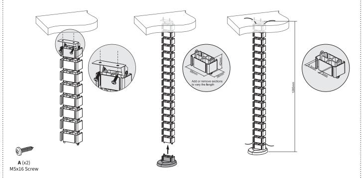
Place the top bracket against the desired location under the desktop and mark drilling locations. Drill 1/4" (6.3mm) deep holes using a 1/8" (3mm) drill bit, then secure the top bracket to the desk using the included screws (A) and a Phillips screwdriver. Assemble the vertebrae sections to the desired length, then insert cables into the corner openings of the vertebrae sections.
